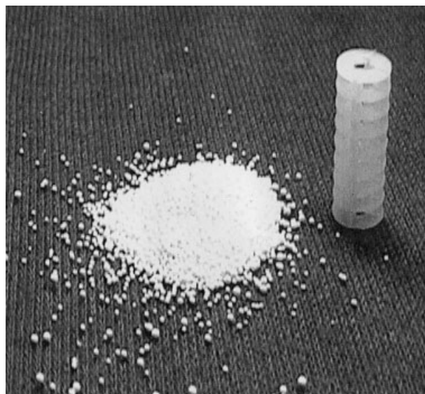
Figure 1 Comparison between a lantern and the amount of resin required to obtain the same loading.
